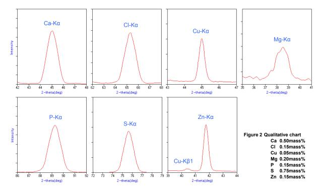
Qualitative scans of each analyte element are shown in Figure 2 and demonstrate the excellent signal-to-noise and spectral resolution of the wavelength-dispersive technology in the Rigaku Supermini200.
